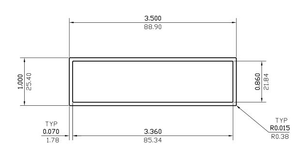
0.070 (1.78) WALL THICKNESS EXCEPT AS SHOWN DATE REV DESCRIPTION BY 03/14/23 REMOVED ALLOY NDZAL мм.2 393.809 0.610 IN.<sup>2</sup> EST.AREA EST.AREA 1.072 0.720 EST.WT. LBS/FT. EST.WT. KG/M. 17.388 441.668 EST.PER. MM. EST.PER. 8.974 227.9 OUT PER. OUT PER. MM. 3.632 92.251 C.C.D. C.C.D. MM. FINISH M/F ALLOY DWN BY P.M.FACTOR 24 SCALE 1:1 DATE 05/30/2011 CKD BY
